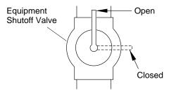
Figure 13 - Equipment Shutoff Valve
